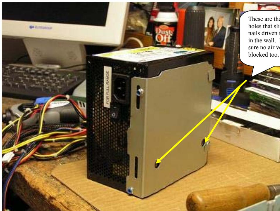
**Figure 9 Custom bracket made to hang the PSU on the wall**
