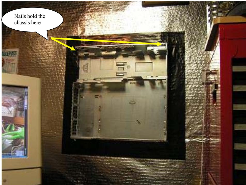
**Figure 3 Mounting the chassis to the wall with two nails**
