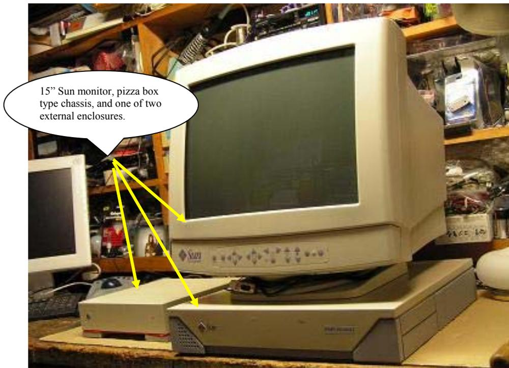
**Figure 2 Original Sun X-Terminal with monitor and external SCSI drive case**
