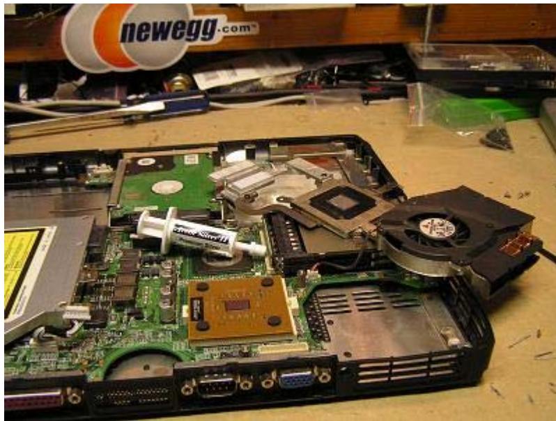
Figure 10 Removing the CPU cooler and applying fresh thermal interface material
