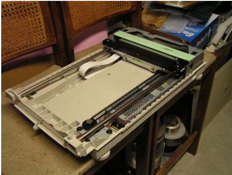
Figure 2 The interior of the HP 6100C scanner
