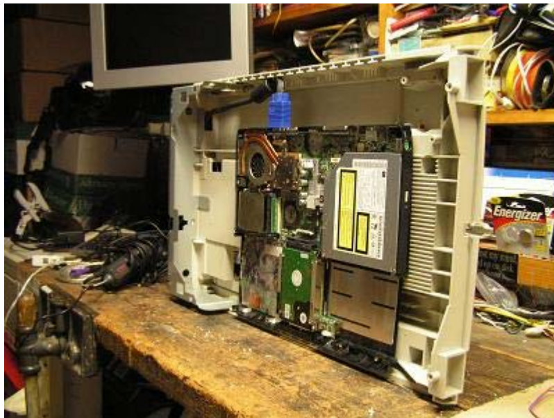
Figure 11 Mounting the laptop to the scanner cavity with three bolts
