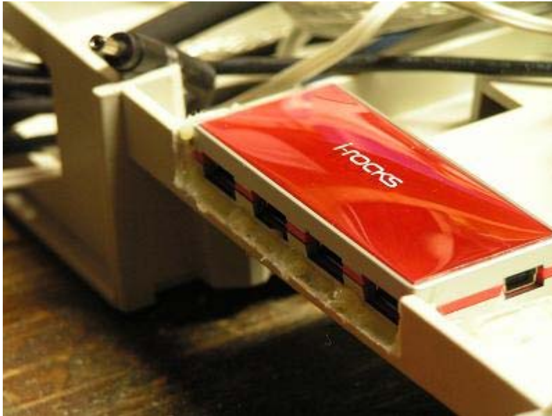
Figure 12 Mounting a USB 2.0 hub with the hot glue gun
