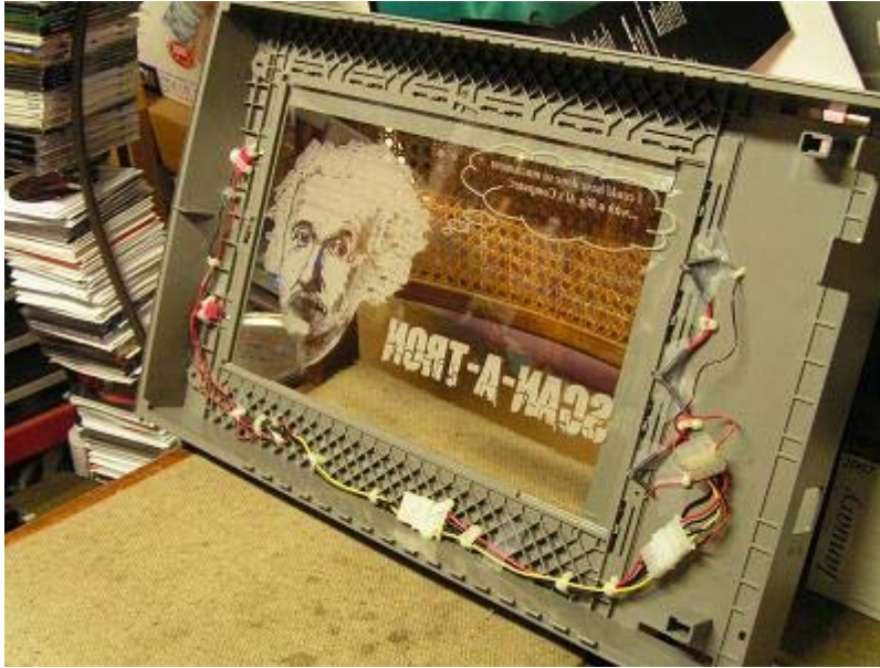
Figure 8 Mounting LEDs along opposite edges of the laser-etched window
