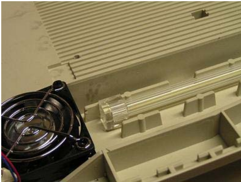
Figure 9 Mounting 12" cold cathode tubes within the scanner cavity
