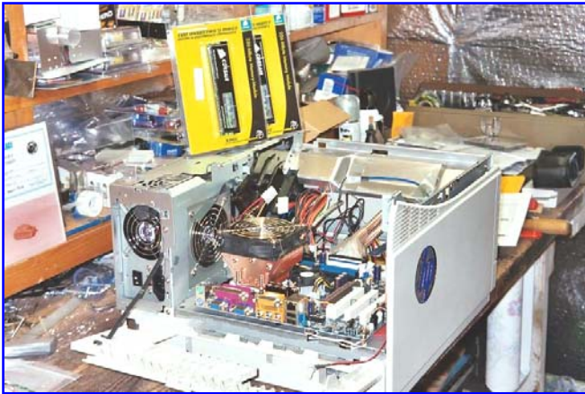
Figure 6. With the motherboard installed, it's time for the XMS memory.
