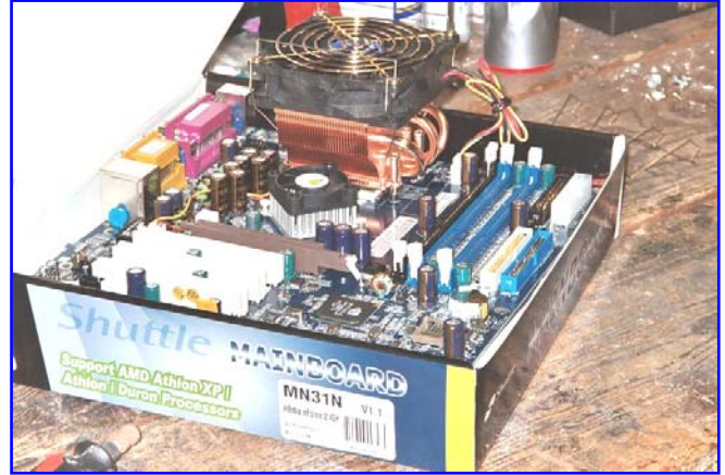
Figure 5. The Shuttle motherboard with the Thermalright SP-97 heatsink.
