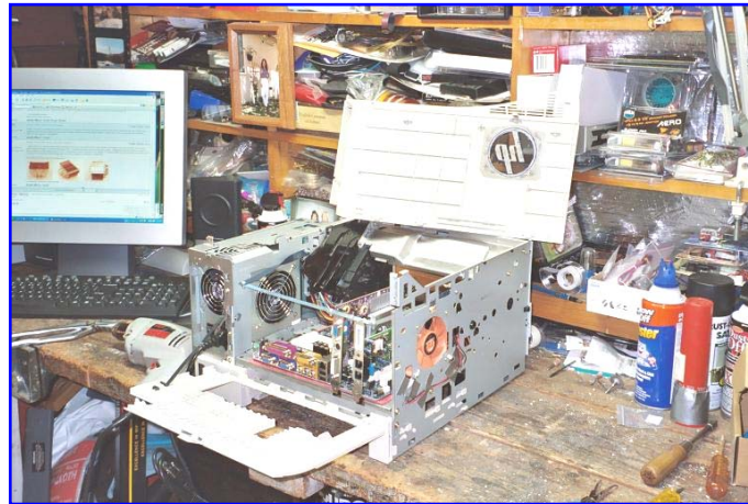
Figure 3. Hacksaw blades form the upper support for the AGP and PCI cards.
