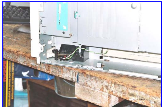
Figure 9. I used the existing rocker switch to activate the PC power switch.
