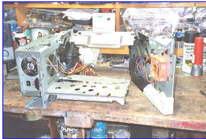
Figure 2. Fabricating a new base for the motherboard.
