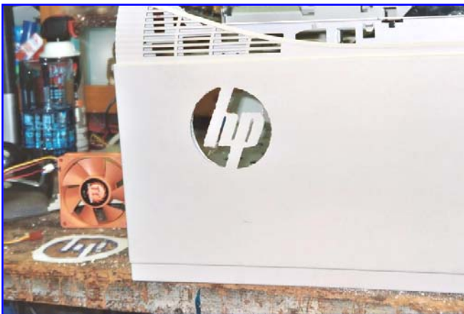
Figure 8. After creating a stencil, I used a Dremel to cut out the HP logo.
