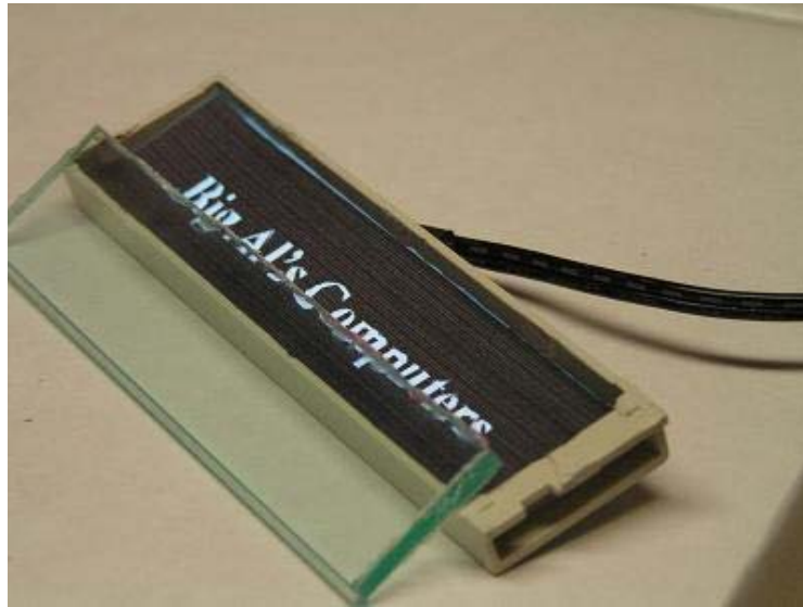
Figure 9 Cover Plate to Keep the Paper Logo Flat Against the EL Panel
