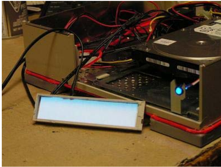
Figure 6 The EL Panel Still Works After Trimming
