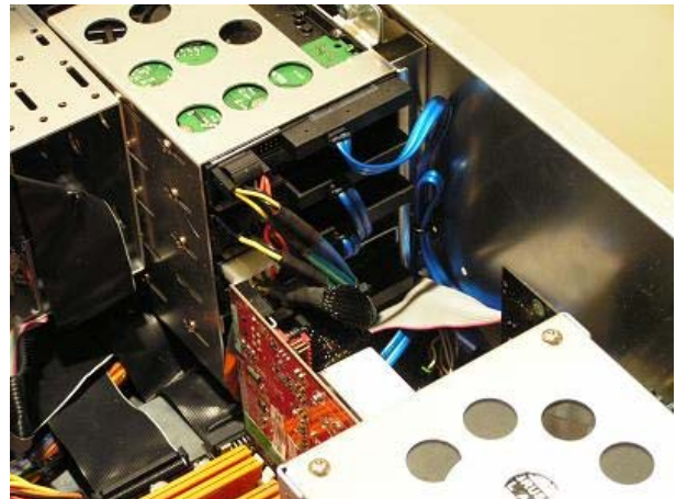
Even the SATA cables and Molex power connectors are tucked away.
